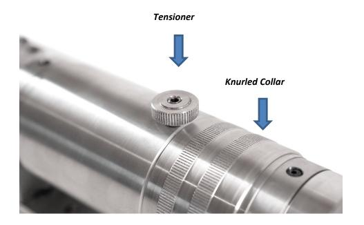
1.Move the barrel clockwise to tighten the shifter feel2.Move the barrel anti-clockwise to loosen the shifter feel
