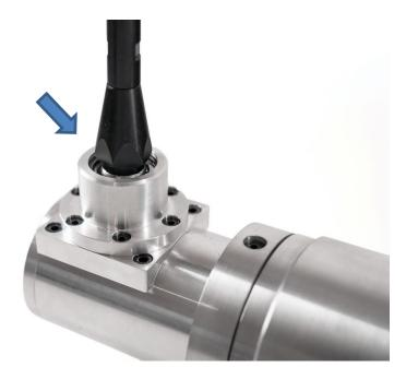
If it looks like the lubrication has dried, the ball joint feels rough or it has been over a year since last adding lubrication after regular use, we recommend smearing a tiny amount (half a pea) lithium-based grease onto the top of the joint and moving through the gears so the parts all get a coating.
